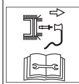
Switch the machine off prior to any work, such as adjustments, cleaning, testing and pull the spark plug.
